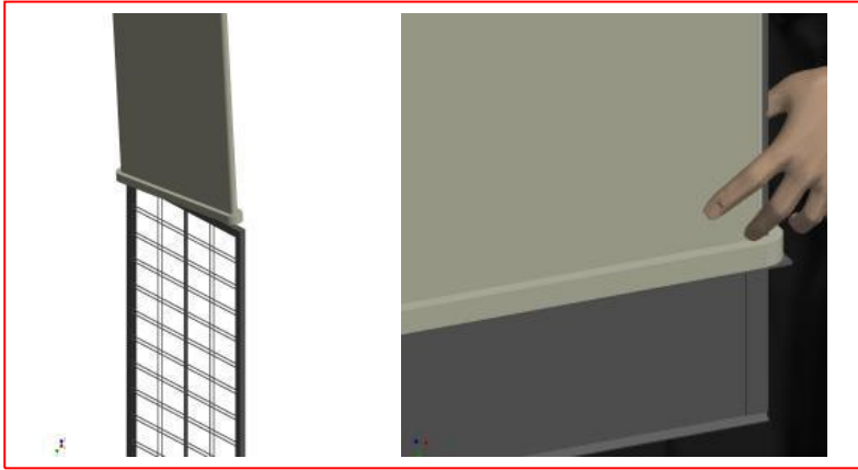
Fig.6- Place the bag in the cage
