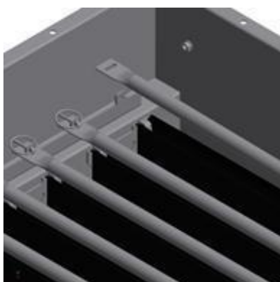
Fig.4 -Remove blowtube
