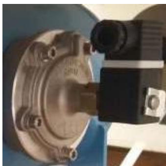
* Fig.10 diaphragm -Valve
